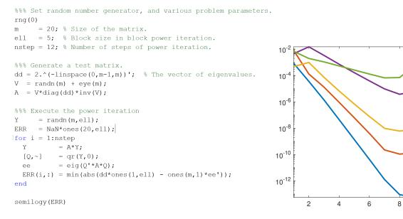
(a) The reason convergence quickly stops is that round-off errors aggregate at every step. Insert the line  $[\mathbf{Y}, \sim] = \operatorname{qr}(\mathbf{Y}, 0)$  immediately after the line with the for command. Then rerun the experiment. Hand in a figure of the new convergence plot.
