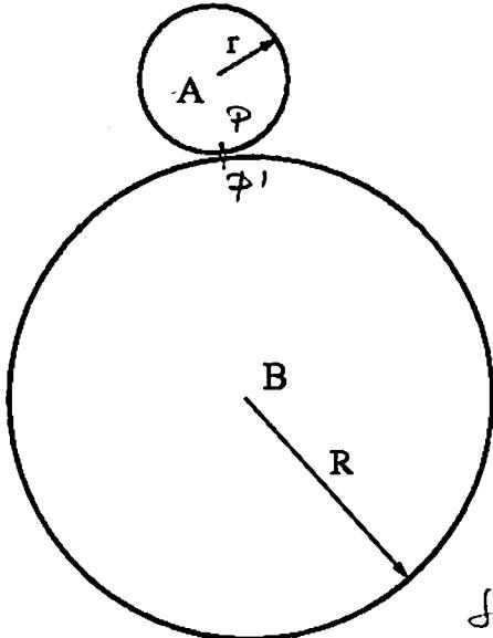
$$T = \frac{1}{2} m v_A^2 + \frac{1}{2} \underbrace{\left( \frac{1}{2} m r^2 \right)}_{I_A} \omega^2$$
