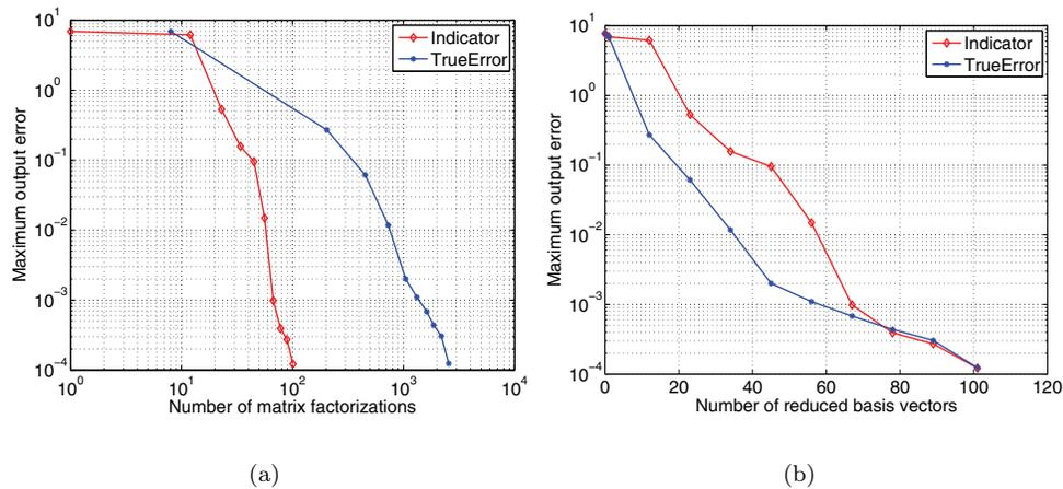
FIG. 5.4. Error indicator versus true output error for the thermal fin with 21 parameters. The same sequence of initial guesses is used for both true-error and error-indicator approaches, and the Gram–Schmidt procedure is used to update the reduced basis.
