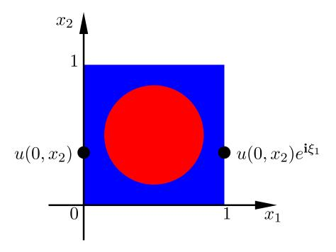
The wave propagation problem in the infinitely repeating unit cell is formulated as a Helmholtz problem with periodic boundary conditions:
