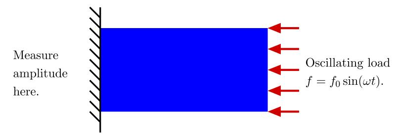
Design the blue box so that the amplitude of the vibration at the attachment point is minimized.
