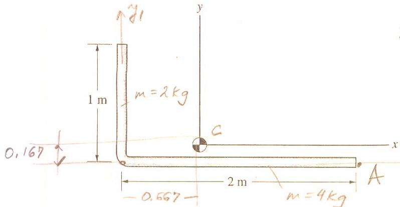
$g = \text{const} \Rightarrow$  center of mass coincides with the centroid
