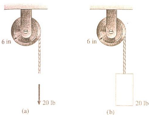
In the second. Forces are identical but the inertia is bigger.
