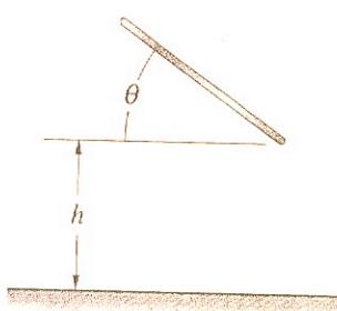
Stage 1 : Free fall , use the work and energy principle
