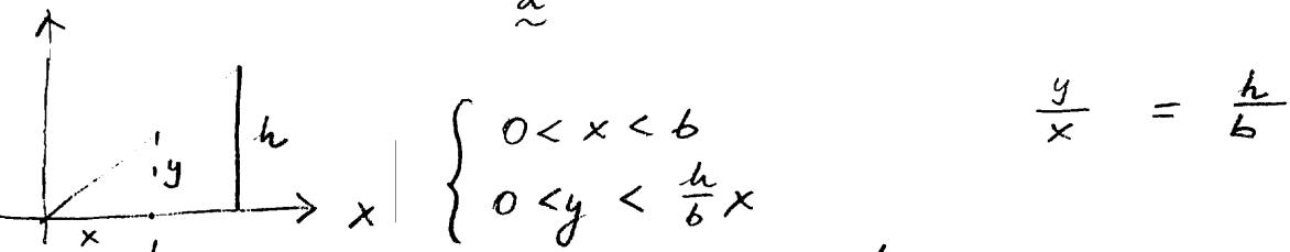
$$I_x = \int_0^b \int_0^{\frac{h}{b}x} y^2 dy dx = \int_0^b \frac{y^3}{3} \Big|_0^{\frac{h}{b}x} dx$$
