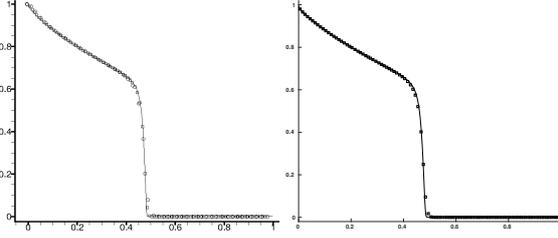
Figure 16: Buckley-Leverett equation with initial condition (58) at time  $t = 0.2$  on a non-uniform mesh. On the left are results for explicit SSP2-3-4 with  $\Delta t$  satisfying  $\max_u |b'(u)|\Delta t/\min_i h_i^2 = 0.25$ , and depicting with circles for  $M = 50$  and squares for  $M = 100$ . On the right are results for implicit Radau3-3-4 with  $\Delta t = h$ . The solid lines are the reference solutions with  $N = 800$  (explicit) and  $M = 400$  (implicit).
