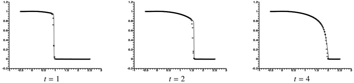
Figure 19: Moving glacier on a uniform mesh of  $M = 100$  elements at various times  $t$ . Circles show the explicit SSP2/WENO5/WENO-AO(4,3) scheme and squares show the explicit SSP3/WENO7/WENO-AO(6,4) scheme, using  $\Delta t = 5\Delta x^2$  and  $\Delta t = 6\Delta x^2$ , respectively. The solid line is the reference solution (the latter scheme with  $M = 800$ ).
