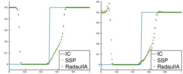
Figure 8: Buckley-Leverett problem. Comparison of the implicit SSP3/WENO-AO(3,2) scheme and the implicit Radau3-3-4 scheme, using a nonlinear mesh of  $M = 100$  elements. On the left,  $\Delta t = 0.5h$  (SSP is stable) and on the right,  $\Delta t = 2h$  (both unstable).
