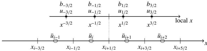
Figure 3: Reconstruction of  $b(u)$  on the big stencil. The data  $\bar{u}_{i-1}, \bar{u}_i, \bar{u}_{i+1}, \bar{u}_{i+2}$  is fit to a polynomial  $P(x)$ , which is evaluated at the uniformly distributed local points  $x^j$  to define  $u^j = P(x^j)$ ,  $j = -3/2, -1/2, 1/2, 3/2$ . Then  $b_j = b(u_j)$  are point values of  $b$ , which are fit to a polynomial  $Q(x)$ .
