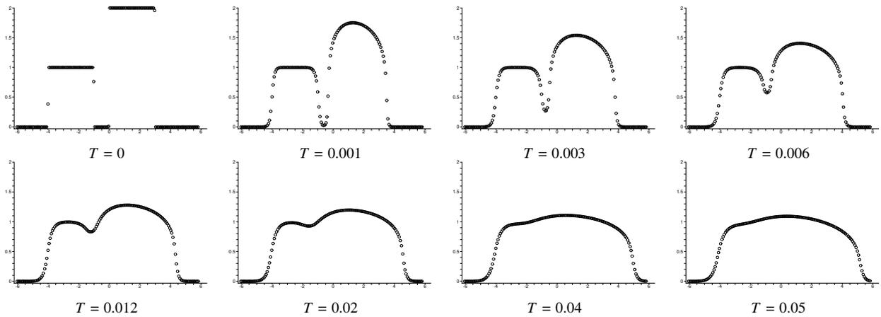
Figure 13: PME collision of two boxes with different heights for  $m = 6$  using an  $x$ -dependent diffusion on a non-uniform mesh of  $M = 160$  elements for the explicit SSP2-3-4 scheme, with  $\Delta t$  satisfying  $\max_u |b'(u)|\Delta t / \min_i h_i^2 = 0.25$ .
