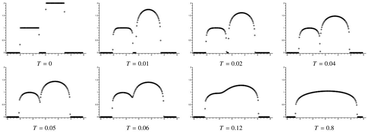
Figure 11: PME collision of two boxes with different heights for  $m = 6$  on a non-uniform mesh of  $M = 160$  elements for the explicit SSP2-3-4 scheme, with  $\Delta t$  satisfying  $\max_u |b'(u)|\Delta t / \min_i h_i^2 = 0.25$ .
