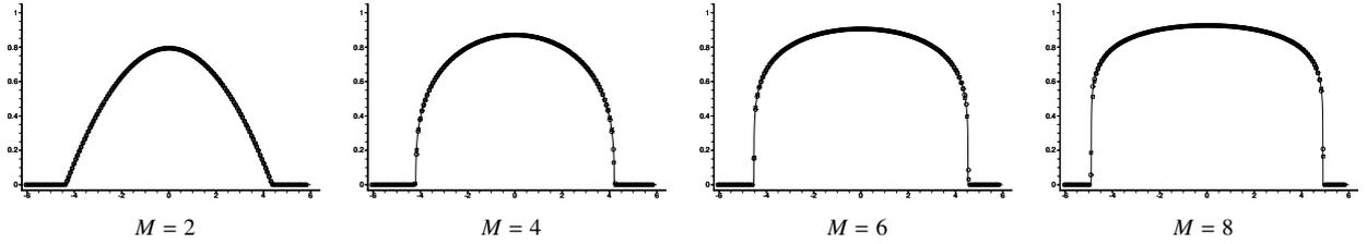
Figure 9: Barenblatt solution of the PME on a non-uniform mesh of  $M = 160$  elements at time  $t = 2$ . Circles are for the explicit SSP2-3-4=SSP2/WENO(3,2)/WENO-AO(4,3) scheme, squares are for SSP3-5-6/WENO(5,3)/WENO-AO(6,4), using  $\Delta t$  satisfying  $\max_u |b'(u)|\Delta t \min_i h_i^2 = 0.35$  and  $\max_u |b'(u)|\Delta t / \min_i h_i^2 = 0.4$ , respectively. The solid line is the exact solution.
