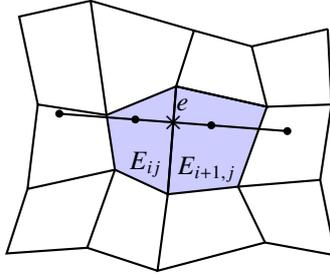
Figure 6: The sampling line and sample points used for logically rectangular WENO-AO(4,3) reconstruction of the diffusive flux. For the quadrature point, shown as a cross ( $\times$ ), on the interface  $e$  between  $E_{ij}$  and  $E_{i+1,j}$ , the sampling line goes through this point and is perpendicular to  $e$ . Sample points, shown as dots, are taken on this line. In any dimension (two space dimensions are depicted), the local computational mesh is one dimensional.
