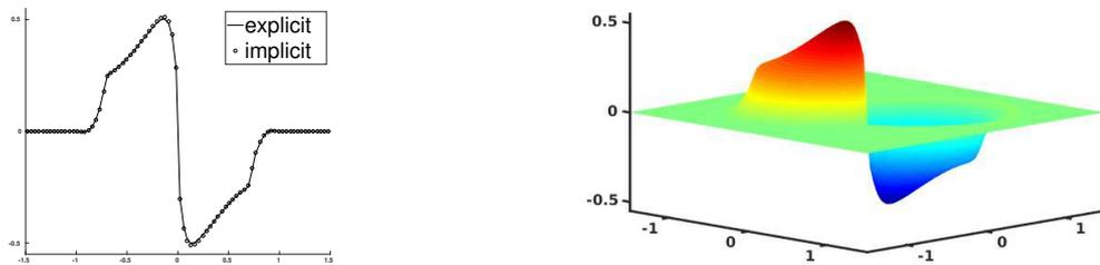
Figure 22: Burgers equation in 2D with a discontinuous diffusion coefficient. Solutions using  $M = 80$  quadrilateral elements at time  $t = 0.5$ . A cross-section of the results for both the explicit ( $dt = 2h^2$ ) and implicit ( $dt = 4h$ ) schemes (left), and the implicit solution (right).
